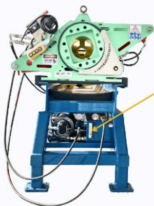
SPU, Standard power unit for HTW50 Slides under the table
