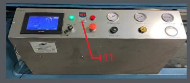
The control panel contains the touch screen, the adjustments for the drive travel pressure, drive travel speed, and the honing head rotation speed. The control panel also includes gauges for the different settings, including the honing fluid pressure and the hydraulic pump pressure.
