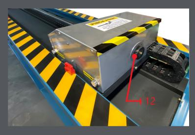
The PLC and the patent-pending constant-torque clutching mechanism is the key advantage of the HONIX 15/20 that allows the operator free to perform other shop tasks while waiting for the honing process to complete.
