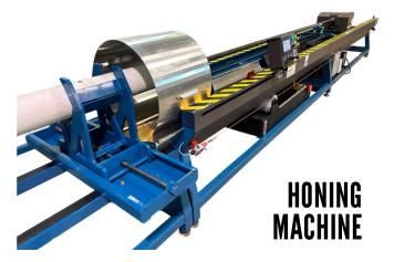
Model Honix15: Max diameter 21", Stroke max 15 Ft. Model Honix20: Max diameter 21", Stroke max 20 Ft.
